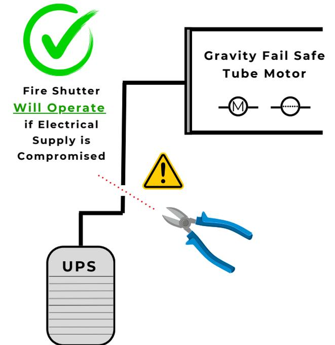
The Gravity Fail-safe motor has been tested and successfully passed to **BS EN 1634-1** at WarringtonFire. Under current regulations **BS EN 16034**, this motor can only be included within a fire shutter/fire curtain that has been tested with that motor type. Other manufacturers of fire shutters will still be required to have an additional test to use this component of a fire application.
